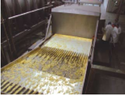
The product falls directly from the cutting line onto the infeed shaker, which spreads the product uniformly and evenly.
